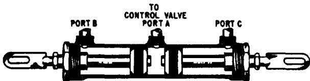
Figure 10-7.—Three-port, double-acting actuating cylinder.
